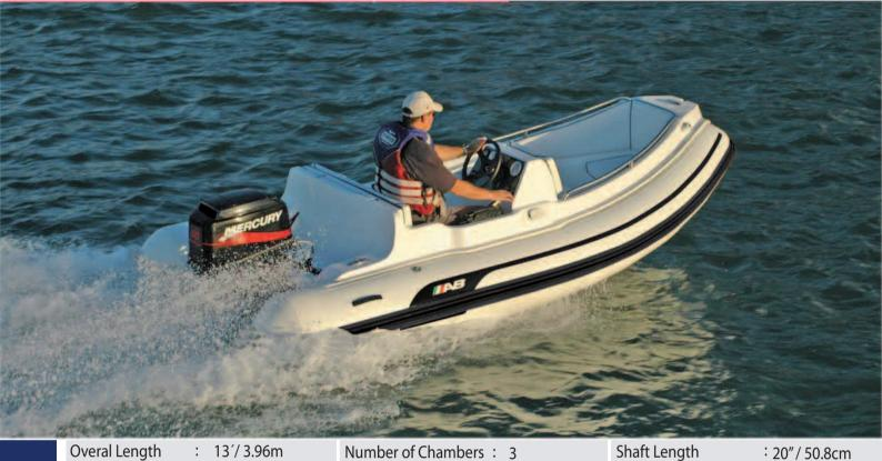
Overal Length : 13'/3.96m Number of Chambers: 3 **Person Capacity Overal Beam** : 6'5"/ 1.95m RDC Design Category : C Inside Length Weight : 9'9"/ 2.97m : 579lb / 263kg Inside Beam Recommended HP : 3'1"/ 0.94m : 40hp / 29.8kw
